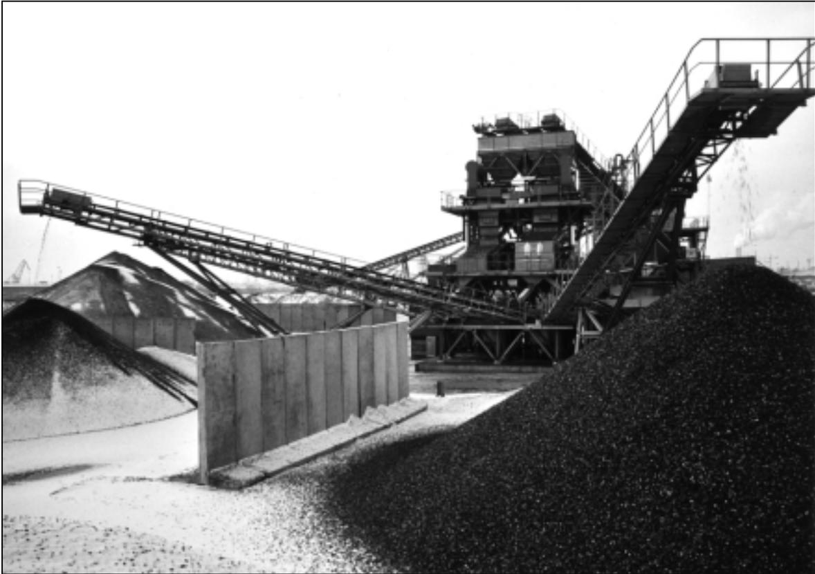
Fig. 11: Gravel scrubbing and separating machine
